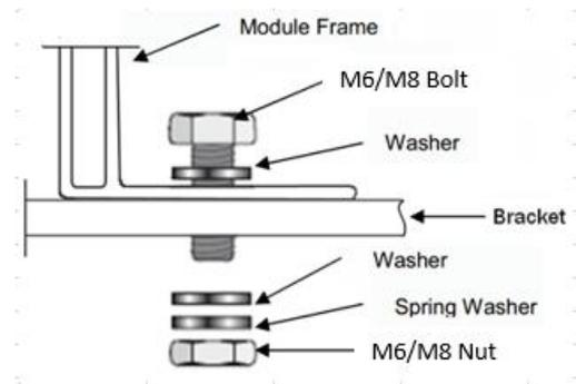
Fig. 2 Diagram of the bolt installation process
